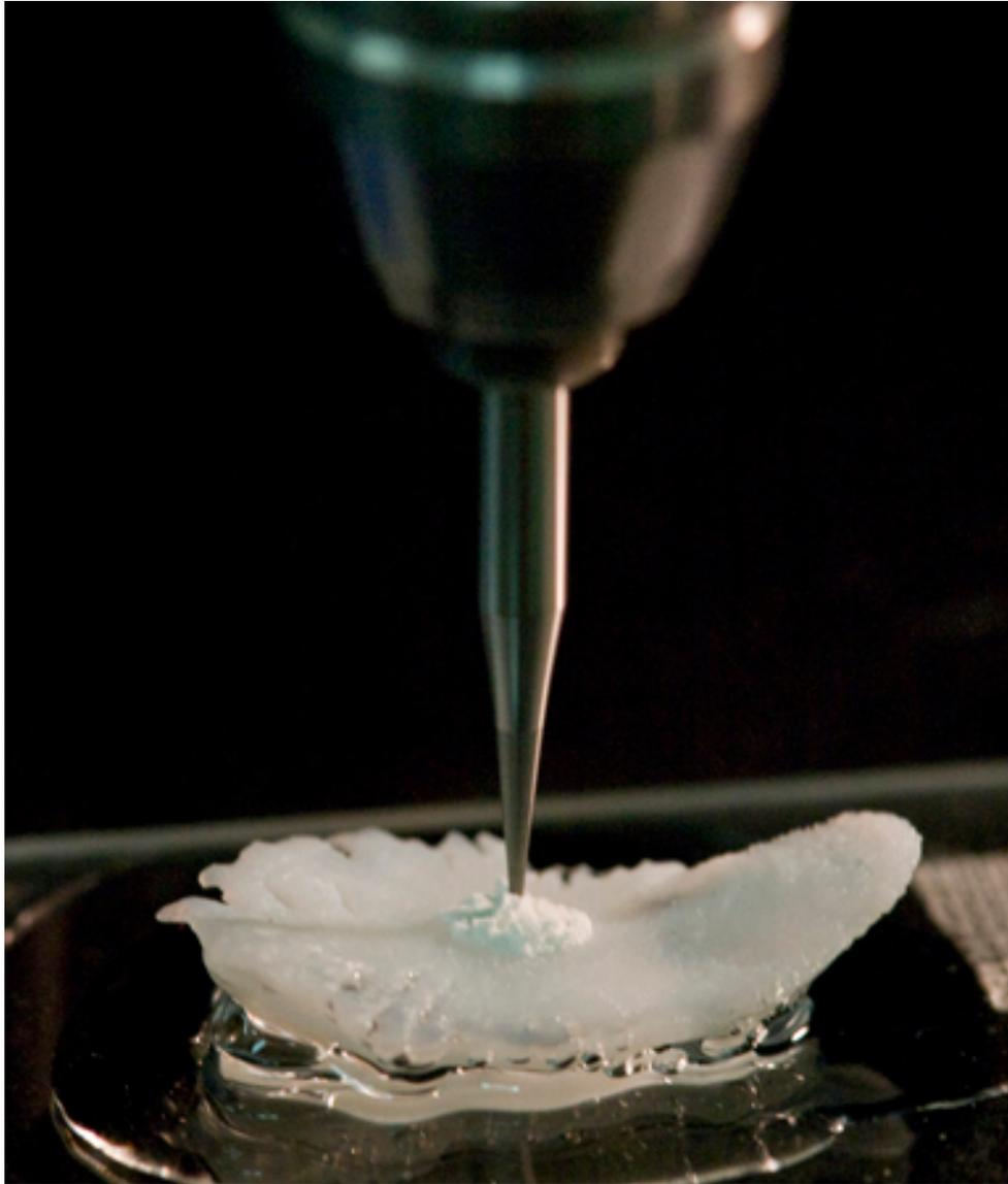
**Figure 11.--Otolith core extraction using the micromilling machine. The small pile of carbonate powder at the surface was analyzed for  $\Delta^{14}\text{C}$  and was typically 3 mg of core material.**
